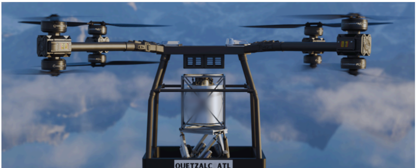
Supratika H13 in flight, instrument payload carried inside the protective cage on the aircraft centreline.
