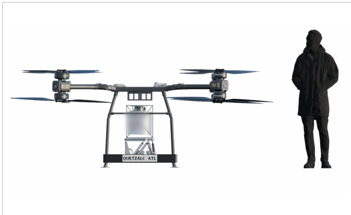
Supratika H13 against a 1.8 m figure. Overall span 3648 mm tip-to-tip; the aircraft transports with the arms folded.
