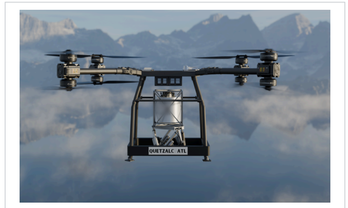
Front elevation. The payload sits on the centreline between the landing gear, below the rotor plane and inboard of the downwash-loaded structure.
